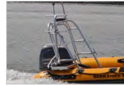
Antenna arch with dive ladder
