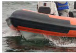
Reinforced tube at bow
