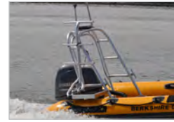
Antenna arch with dive ladder
